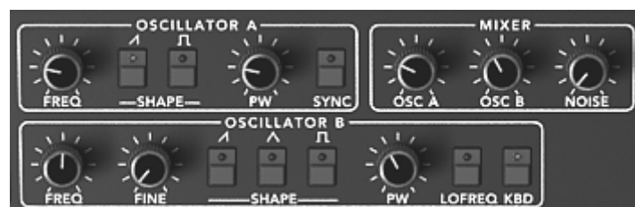
Oscillator Section on the Prophet 5
