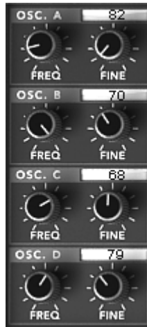
Oscillator Section on the Prophet VS
