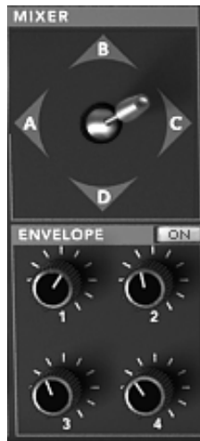
The Mixer of the Prophet VS and its envelope
