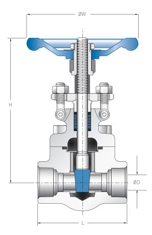
Dimensions for bolted and welded bonnet, reduced port OS and Y gate valves with screwed and socket weld ends.
