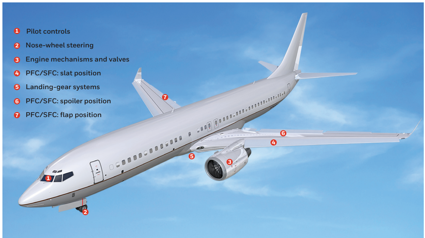
Figure 1. LVDT Position Measurement Applications for Aircraft
