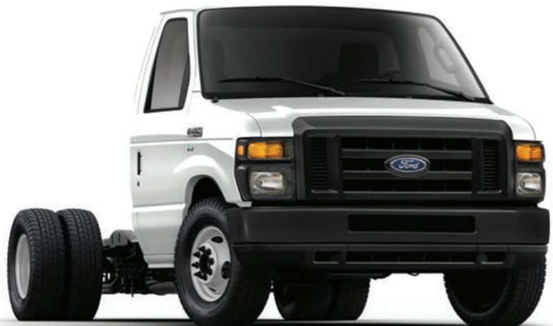
Left: The Class B motorhome is often built on newer Euro-styled vans, like this Ford Transit. Several different roof heights are available from the OEM. Above: The van cutaway chassis features the van cab up front, but a stripped chassis behind.
