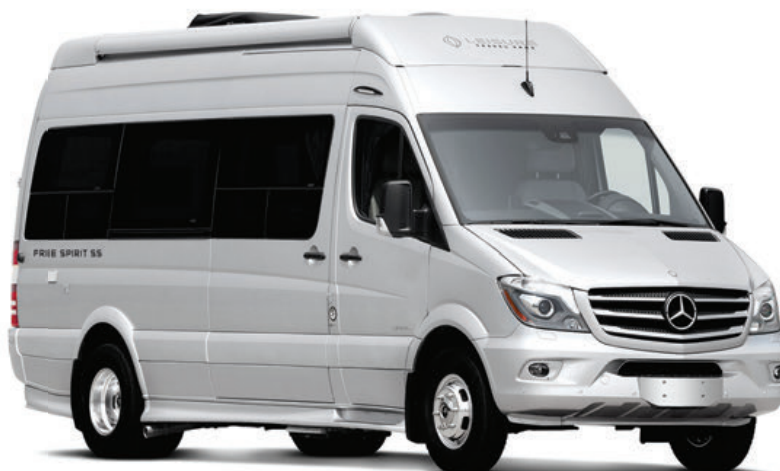
The Class B motorhome is generally built within the confines of a standard panel van, but frequently with a raised roof for additional headroom.
