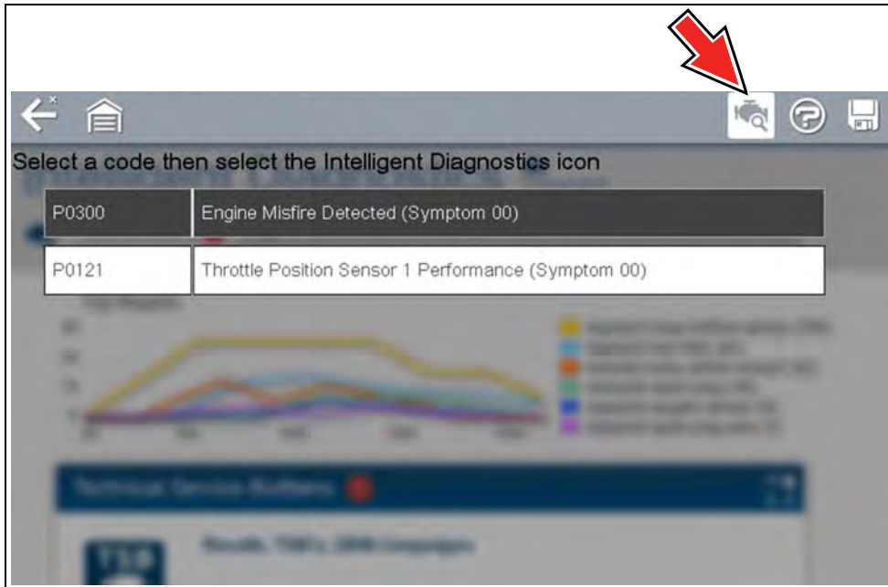
Figure 5-7 DTC results and Diagnose icon
