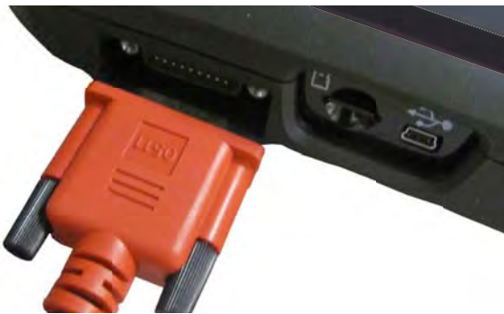
Figure 4-1 DA-4 data cable (26-pin end) connection to diagnostic tool
