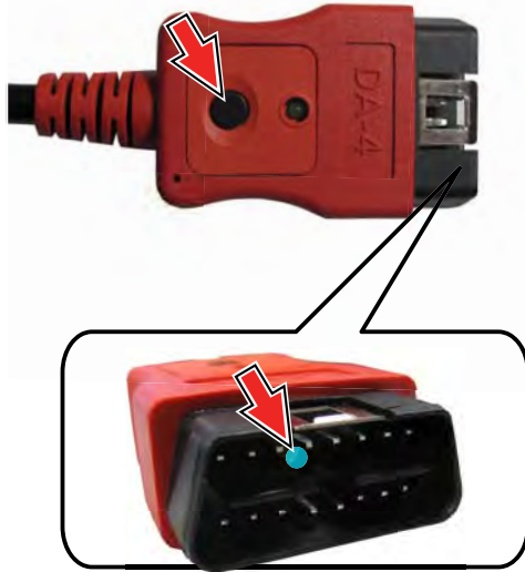
Figure 4-3 DA-4 data cable LED flashlight
