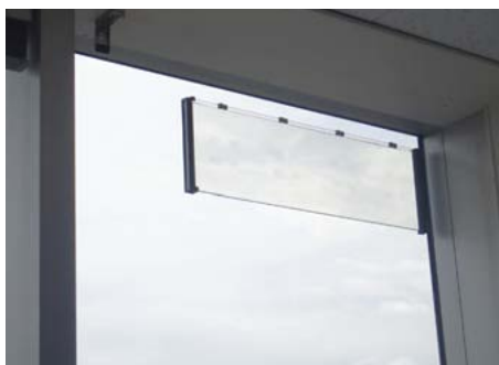
Glass antenna attached to an existing window
