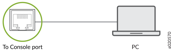
Figure 46: Connect a Device Directly to a Management Console
