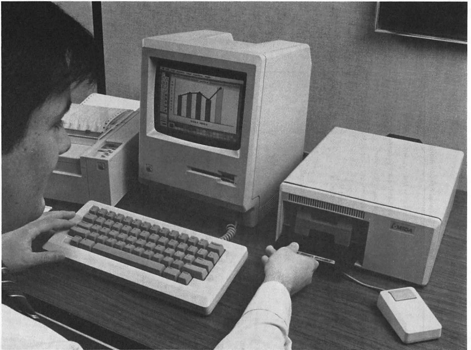
7 Fig. 2-1. A Macintosh system that has been expanded to use an ImageWriter printer and a Bernoulli Box hard disk (courtesy IOMEGA Corp.).
