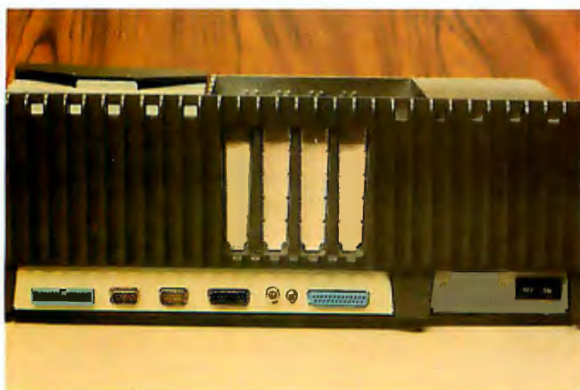
Photo 4: Back view of the Apple III, showing (from left to right) the 26-pin flat-ribbon connector for daisy-chaining up to three additional floppy-disk drives into the computer; two DB-9 connectors for joysticks, etc.; a DB-15 video-out connector with black and white, NTSC color (the standard North American color-television system), and RGB (red, green, blue); an RCA-type video-out connector (for black and white only); an external speaker jack; and an RS-232C serial I/O (input/output) port for a letter-quality printer, modem, etc.
