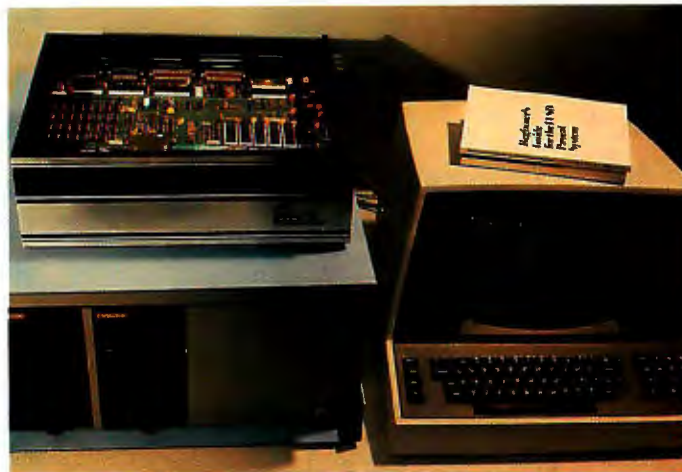
Figure 1: The Pascal Microengine is shown here in a system which includes two Shugart 8-inch disk drives in an Integrand cabinet and a Boroc IQ120 terminal. The computer uses a 16-bit processor chip and it executes p-code directly through the use of three Microengine integrated circuits on which the processor microinstructions are stored. The Microengine also includes 64 K bytes of memory, a 24-bit parallel port, and two RS-232C serial interfaces. The software provided is the UCSD extended Pascal system.
