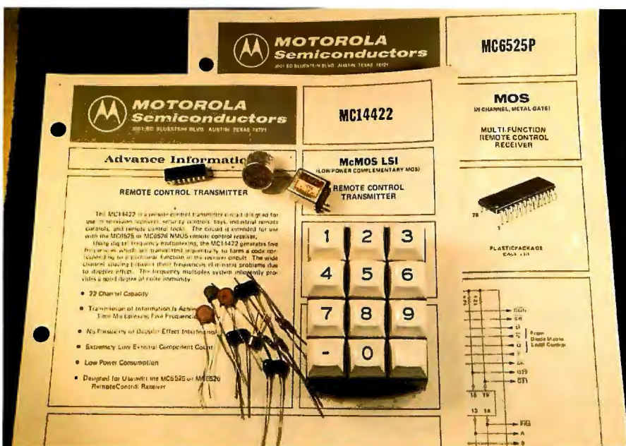
Photo 2: Assembled here are the parts needed to build a remote-control unit that uses the Motorola MC14422 CMOS LSI remote-control transmitter and MC6525 receiver.
