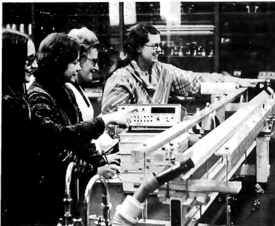
Photo 2: Forensic physics students taking data with a multimemory digital timer and an air track.
