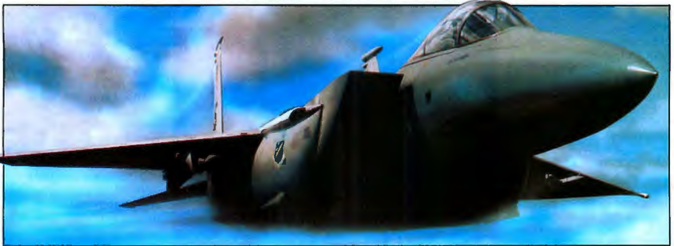
The F-15 served as a test bed for a flight control system written in the Ada language. Ada was designed to meet today's demands for a standard computer language, producing efficient, reliable and maintainable code.
