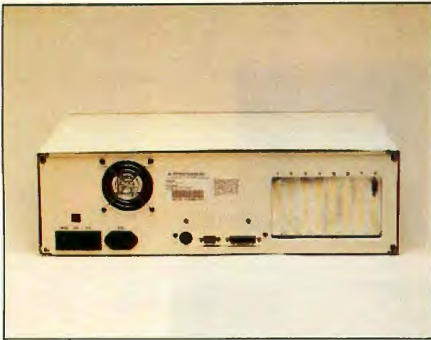
The rear of the Tele-286 showing the power cord receptacle, monitor power cord socket, serial and parallel ports, and access slots for expansion boards with the TeleVideo HRM-100 monitor adapter installed.
