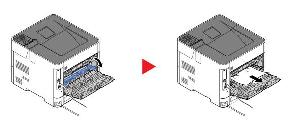
If you cannot find a paper jam, try checking inside the rear of the machine.
