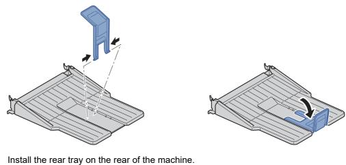
Install the rear tray on the rear of the machine. 2
