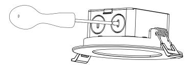
Open the power supply box cover. Feed the supply wire into the knockout hole using a 1/2 in. clamp connector (not included) and make all the connections inside the power supply box using wago connectors. Connect the 120V line (black) wire to the black wire. Connect the neutral (white) wire to the white wire. Connect the ground (green) wire to the green wire. This power supply box needs to be grounded.
