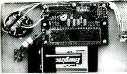
The internal layout of the Tube Amplifier Bias Checker is simple and clean. The most complex wiring is with S1 and the resistors. Note how R1 and R2 are mounted directly to S2.
