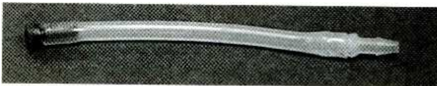
Fig. 3. The core of the air muscle is flexible rubber tubing. One end is plugged with a screw; the other receives an air fitting.
