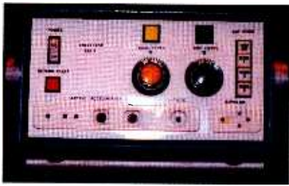
Fig. 1. The front panel of an electrosurgical unit contains the controls that set the power level and mode of operation.
