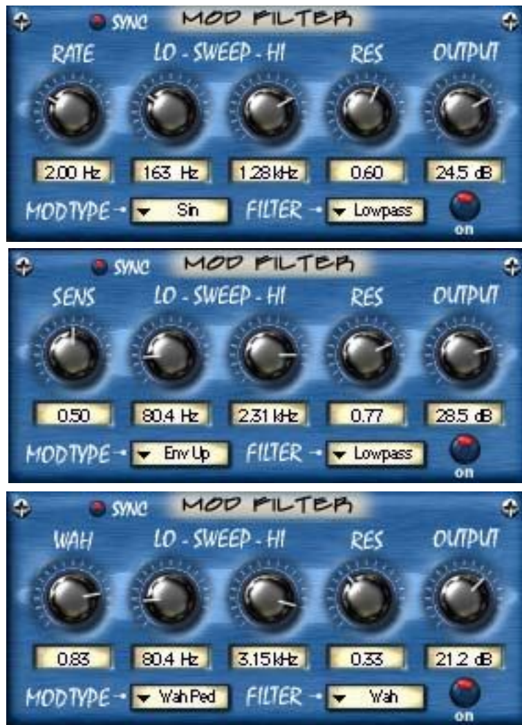
Figure 131. The Mod Filter plug-in window The label and function of the first knob depends upon the Mod Type menu selection.
