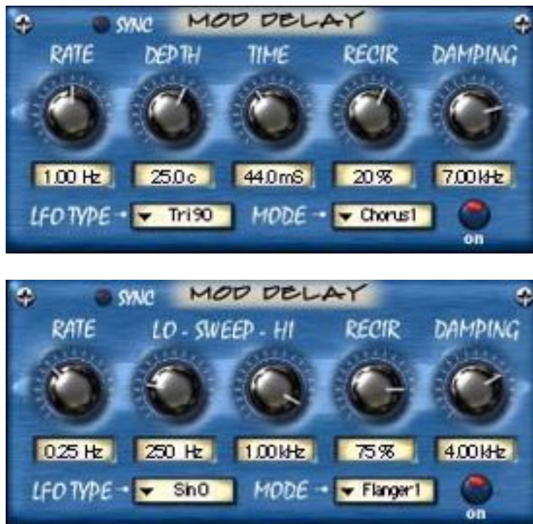
Figure 134. The Mod Delay module The label and function of the second two knobs depend upon the Mode menu selection.
