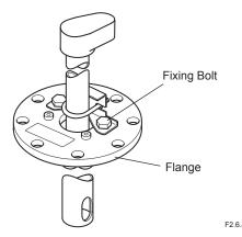
Figure 2.6 Removal of Sensor Holder (for Flange Mounting Sensor without Cleaners)
