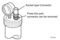
Figure 3.2 Socket Type Connector.
