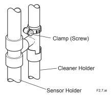
Figure 2.7 Removal of Sensor Holder (with Cleaner)
