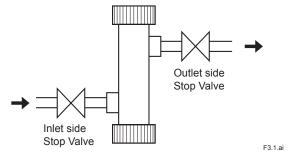
Figure 3.1 Process Piping of Flow-through Type Holder.
