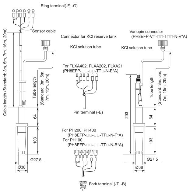
Figure 1.1 PH8EFP Filling type pH Sensor
