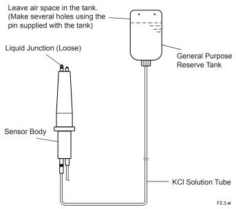
Figure 2.3 Supplying KCI Solution to Sensor Body
