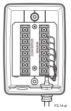
Figure 2.14 Connecting Sensor Cable (In case of the PH8TBG)
