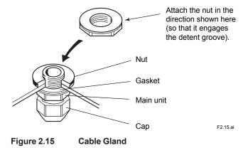
(5) After completing the cable connections, replace the box cover securely, thus preventing moisture from getting into the case.
