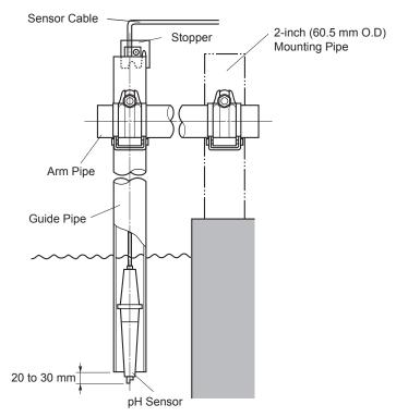
Figure 2.4 Mounting Sensor in Guide Pipe
