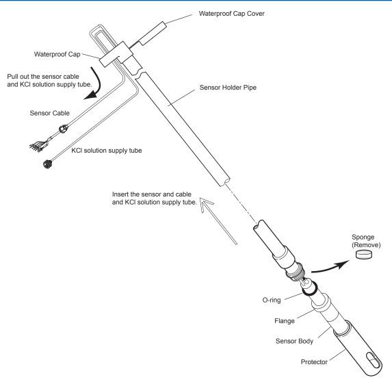
Figure 2.8 Installing the Sensor Cable
