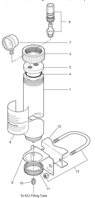
Qty Item Part No. Description K9142VL Tank Assembly 1 Block 2 K9142VJ 3 K9142VK Block 4 G9303AE O-Ring 6 L9835DD Joint L9867BS Pressure Gauge 8 K9142RU Label 9 K9142VP Bracket 10 K9142EJ Сар 11 K9142VQ Ring 12 L9826AL Bracket U-Bolt 13 D0117XL-A
