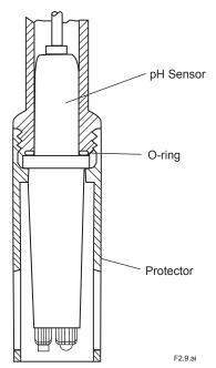
Figure 2.9 Installing Sensor in Submersion Holder
