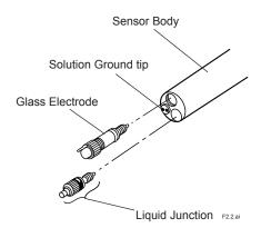
Figure 2.2 Names of PH8EFP pH Sensor Components
