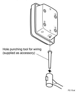
Figure 2.13 How to punch out the wiring hole
