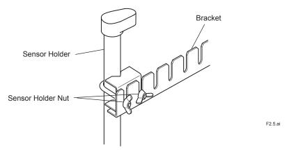
Removal of Sensor Holder (Stainless Bracket used with option /MS3 or /MS4)
