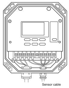
Figure 2.16 Connecting Sensor Cable to Two-wire pH Transmitter
