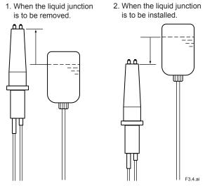
Figure 3.4 Replacing Liquid Junction
