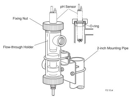
Figure 2.12 Installing Sensor in Flow-through Holder
