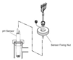
Figure 2.10 Preparation for Sensor Cable Connection
