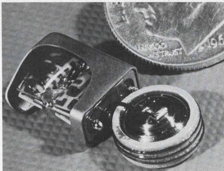
Microminiature temperature transmitter , designed to be implanted in a human body, is said to be capable of detecting temperature changes of 1/100 to 1/1000°C. Developed by NASA's Ames Research Center, the transmitter contains four hybrid integrated-circuit chips mounted inside a hermetically sealed can for protection from body fluids. The circular portion contains the battery and antenna and is usually left outside the body.
