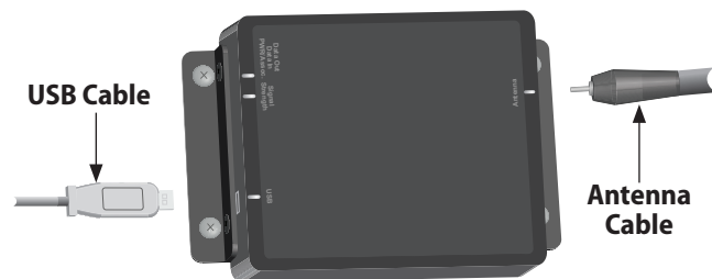
Figure 14 - ISG-2400 Gateway Router Installation
