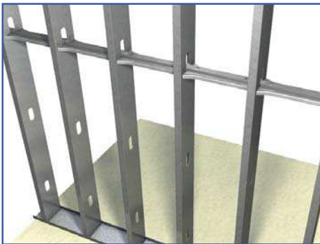
When using BuckleBridge in curtain walls with standard "cee" studs, one screw is only needed every 3rd stud.*
