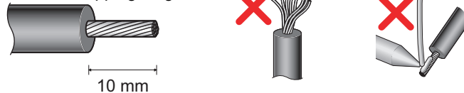
Cable sheath stripping length
