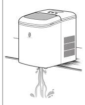
Once completed, drain out the water by unplugging the drain cap.
