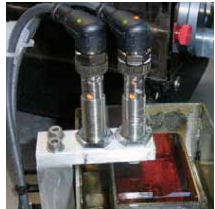
Black, transparent housing for optimum LED visibility.
