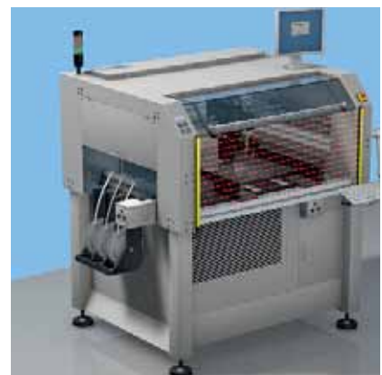
Safety light curtains can be used for finger or hand protection.
