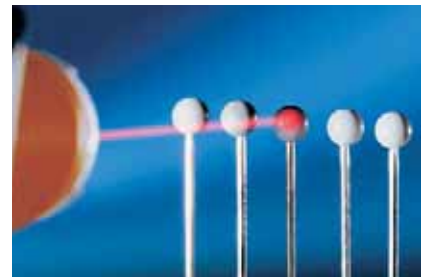
Coherent: Laser sensors emit light of a defined wave length and the same phase position.
