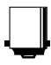
BA 15s DIN: 49720 IEC: 7004-1 I A ANSI: Single contact candelabra bayonet base C81.61-1990 sheet I-20-1
