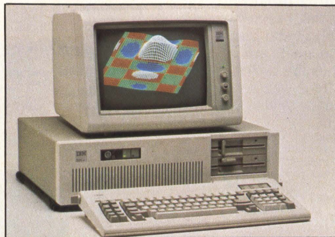
The professional graphics display and adapter, part of IBM's PC/ES technical PC, displays 256 colors from a palette of 4,096, and performs three-dimensional drawing.
