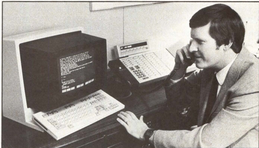
AT&T's System 75 is one of that company's first private branch exchange systems equipped with the Digital Multiplexed Interface, one of two interfaces for connecting terminals and workstations to a host computer via a PBX.
