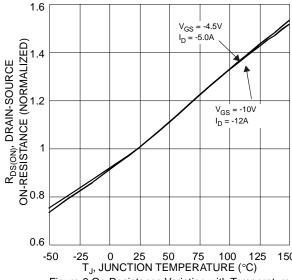
Figure 6 On-Resistance Variation with Temperature
