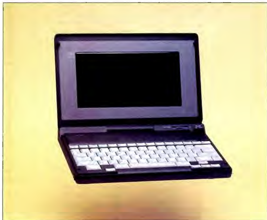
The NEC UltraLite weighs in at only 4 \frac{3}{4} pounds but offers greater performance than an IBM PC XT.
