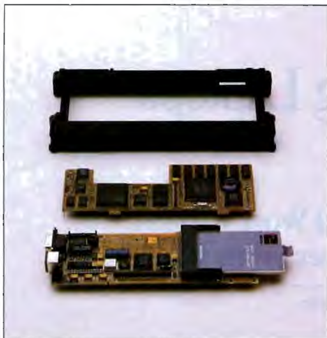
Photo 1: The components of the 80C88 processor slice. Note that the entire 80C88 system fits into a slice about the size of one-third of a piece of paper. The logic board shows a 512K-byte memory card inserted in the memory card slot. The 80C88 system boards feature surface-mounted components and are mounted back-to-back. The primary chip set is manufactured by Western Digital.
