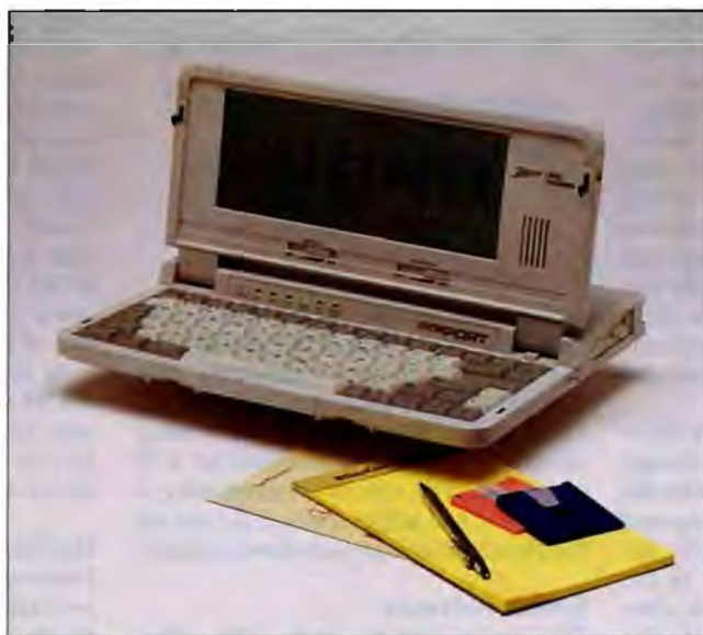
The Zenith MinisPort. The configuration shows the 2-inch 720K-byte floppy disks.
