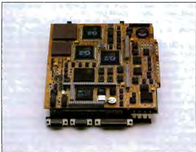
Photo 3: The internals of the 80386 Agilis System. The underside of the board has a bay for a 20-megabyte 2 1/2-inch PrairieTek hard disk drive. The primary chip set is manufactured by Headland Technology. Note the serial and parallel ports at the lower edge.
