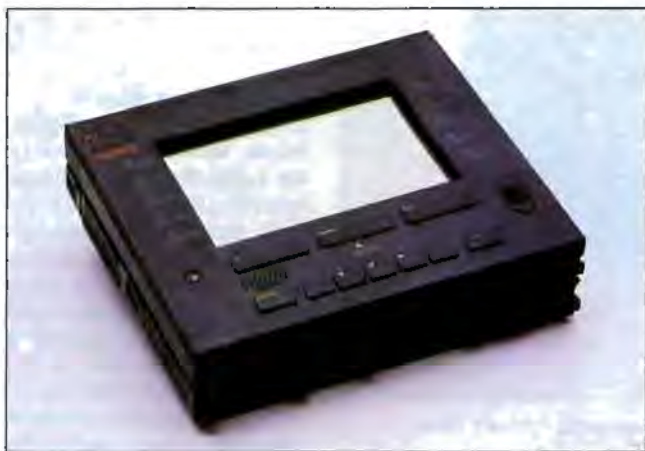
Photo 2: The 80C88 with the touchscreen console slice and a battery pack. This configuration constitutes a complete touch-operated personal computer. Note the programmable function keys around the perimeter of the flat-panel display.
