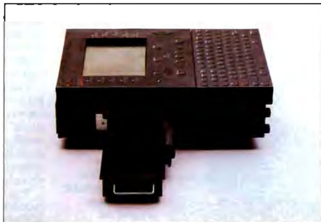
A notebook-size 80386 system showing the console slice, keypad slice, battery packs, and PrairieTek hard disk drive.
