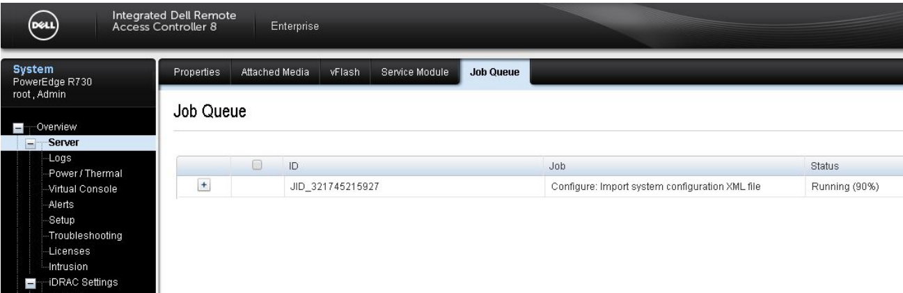
Figure 9 iDRAC8 Auto Config import system configuration job running
