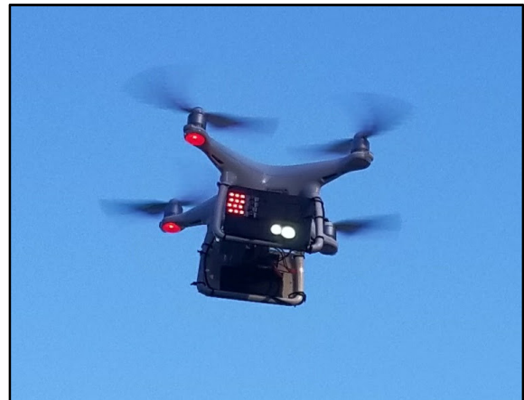
Figure 1: Multiple lighting apparatus being tested for optimizing VLC broadcasts.
