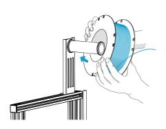
The Nozzle must be hot to add, remove or change filament so preheat the nozzle before starting. Hang the filament spool on the holder so it feeds over the top of the spool towards the extruder..
