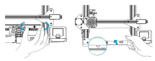
The levelling points are about 30mm in from each corner. There is no need to measure exactly.
