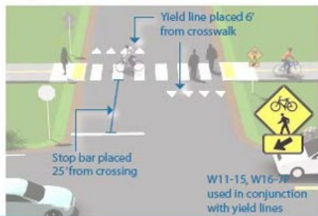
Setback Crossing - A set back of 25 feet separates the path crossing from merging/turning movements that may be competing for a driver's attention.
