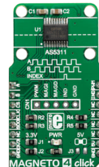
MAGNETO 4 Click The AS5311, a high resolution magnetic linear encoder by ams.
