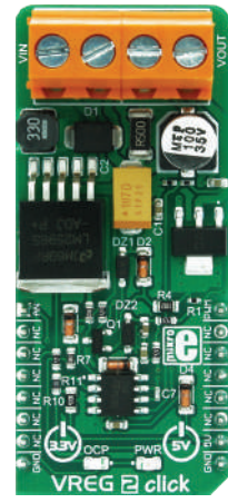
VREG 2 Click Uses the LM2596, a 3A, step down voltage regulator working at 150 kHz, from Texas Instruments.
