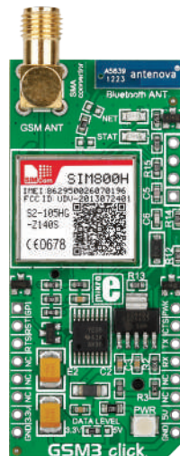
GSM 3 Click With SIM800H quad-band GSM/GPRS module. 85.6 kbps GPRS data transfer.
