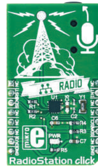
RadioStation Click With the Si4713-B30, the best in class integrated FM broadcast stereo transmitter.
