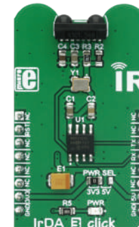
IrDA 3 Click Intelligent IR transceiver device that sends and receives UART commands via the IR interface. MSRP - $26 00 MIKROE-2871
