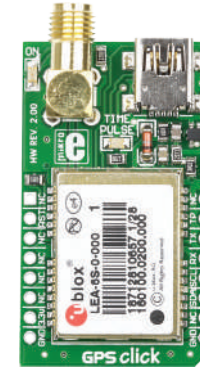
GPS Click It carries LEA-6S high-performance position engine from u-blox.
