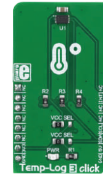
Temp-Log 3 Click Featuring the MCP9843 IC, an accurate temperature sensor IC with integrated EEPROM.
