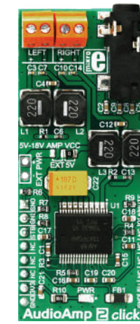
Audio Amp 2 Click The TDA7491, a 20W dual BTL class-D audio amplifier IC, from STMicroelectronics.
