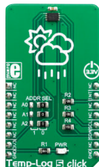
Temp-Log 5 Click Equipped with the CAT34TS02 sensor from ON semiconductor.
