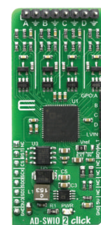
AD-SWIO 2 Click With a 16-bit ADC converter, and 13-bit DAC converter integrated into the AD74413R.
