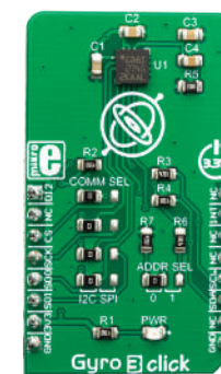
Gyro 3 Click With the I3G4250, a three-axis digital gyroscope.
