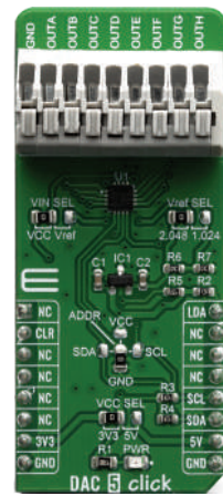
DAC 5 Click It's an advanced 10-bit eight-channel digital to analog converter (DAC) with DAC53608.
