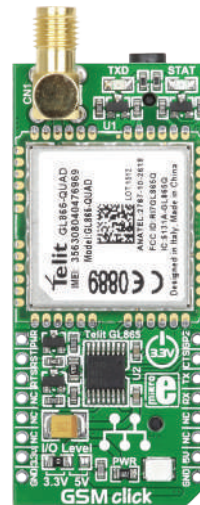
GSM Click With quad-band GL865-QUAD GSM/GPRS module, onboard antenna connector and SIM card socket.
