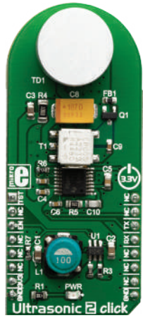
Ultrasonic 2 Click Equipped with the PGA460, a highly-integrated system-on-chip (SoC), based on SONAR principle.
