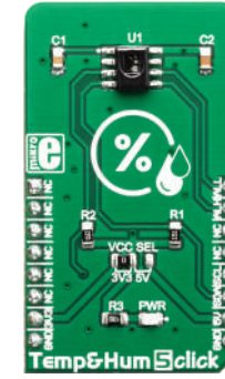
Temp&Hum 5 Click The HIH6130, a relative humidity and temp. sensor with I 2 C Interface, by Honeywell.
