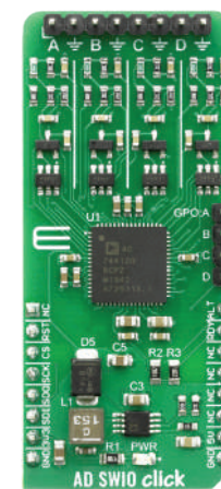
AD-SWIO Click The AD74412R a quad-channel software configurable input/output solution.
