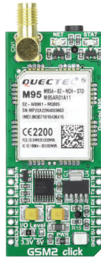
GSM 2 Click With Quectel's M95 FA quad-band GSM/GPRS module. 85.6 kbps GPRS data transfer.
