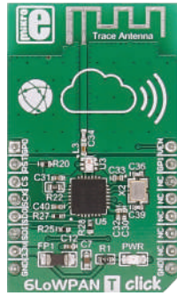
6LoWPAN T Click TI's CC2520, 2.4GHz ZigBee®/IEEE 802.15. RF transceiver.
