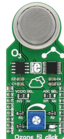
Ozone 2 Click With MQ131 sensor for Ozone [O3]. Detection range 10-1000 ppm of O3.
