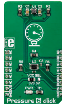
Pressure 6 Click Allows readings in the range from 300hPa up to 1300hPa, with the BM1386GLV sensor.
