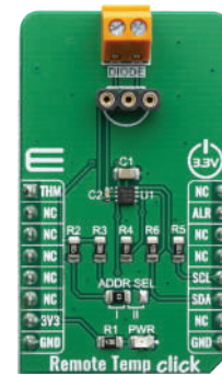
Remote Temp Click The EMC1833 from Microchip, a specifically designed IC, measuring remote temperature.
