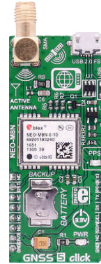
GNSS 5 Click It features NEO-M8N GNSS receiver module from u-blox.
