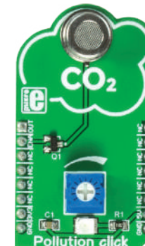
Pollution Click Detects organic gases - formaldehyde, benzene, alcohol, toluene, etc. Detection range 1x50ppm.
