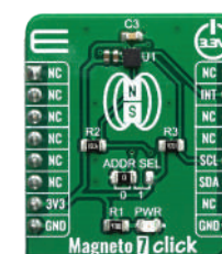
MAGNETO 7 Click The BM1422AGMV, a 3-axis magnetic sensor IC from ROHM Semiconductor.
