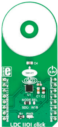
LDC 1101 Click With the LDC1101, the integrated, high-res, high-speed, inductive-to-digital converter.
