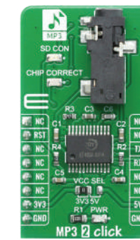
MP3 2 Click Based on KT403A, a hardware audio MP3/WAV decoder and DSP, with on-board microSD card slot.
