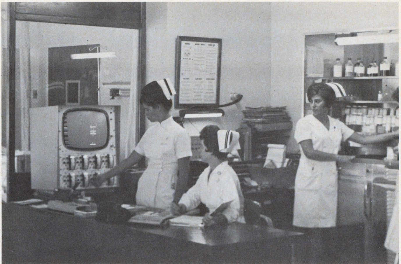
Eight coronary patients can be monitored simultaneously with this intensive-care system installed at the Orange County General Hospital in Orange, Calif. Individual electrocardiograms and other heart parameters can be dis-
