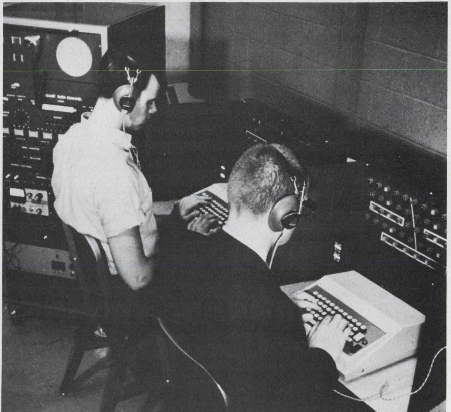
Computer-controlled Morse code training system will let the Army give individualized instruction to 24 students at once. The system is being tested here by its maker, Sylvania Electric Products, Inc.
