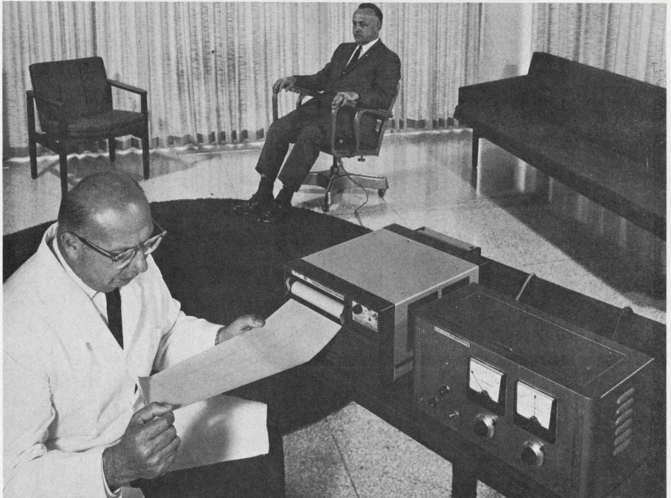
11. Instrumented chair can monitor physiological parameters without the need for attached sensors. Developed by the WDL Div. of Philco-Ford, the technique might also be
