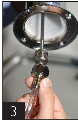
3 Thread beer line connector to draft arm and secure draft arm to cabinet with rubber gasket under the draft arm.
