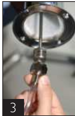
3 Thread beer line connector to draft arm and secure draft arm to cabinet with rubber gasket under the draft arm.
