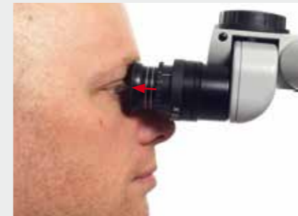
Figure 1.12a Viewing without eyeglasses: screw out the eyecups until 2-3 silver rings are visible
