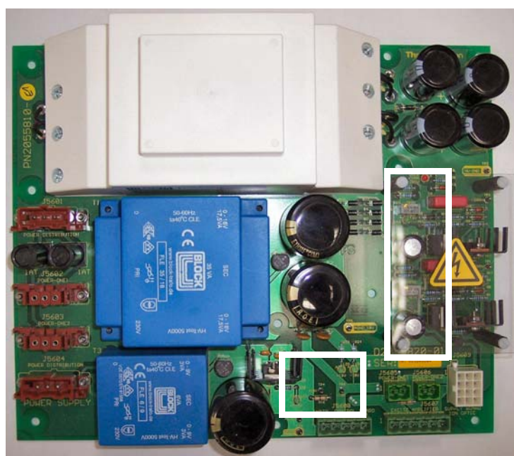
Figure 1-42. Power Supply 1 board
