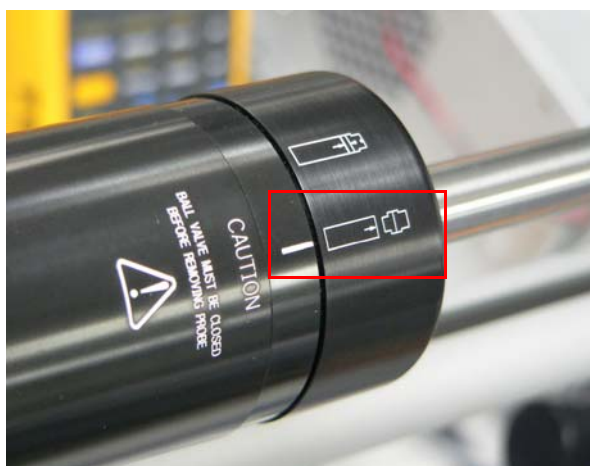
Figure 3-15. Ion volume tool handle in the unlock position
