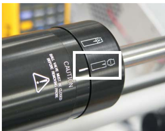
Figure 3-25. Ion volume tool handle in the unlock position
