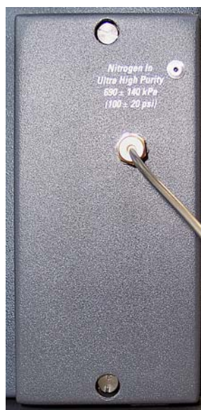
Figure 1-31. ETD reagent carrier gas port at the ETD Module
