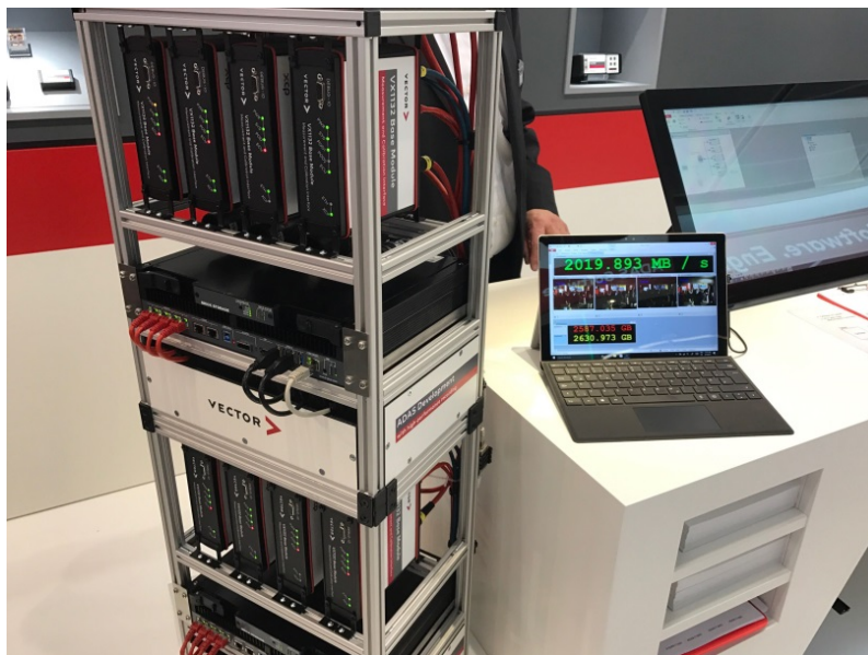
Figure 10: Setup with aluminum frame, the green number on the table shows the current write rate of 2019.893 MByte/s
