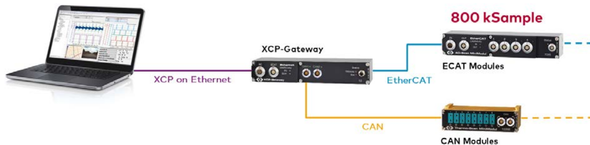
Figure 13: Example of a measurement with 800 kHz sampling rate with CSM modules
