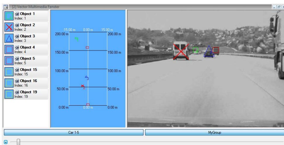
Figure 19: Video display of a reference camera in CANape with overlaid objects that are detected by sensors. Display from a bird's eye perspective and the video image.
