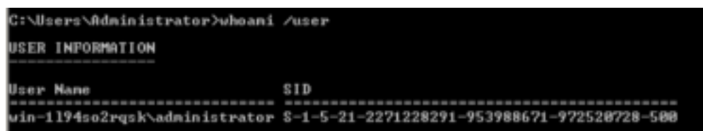
Figure 4-10 ECS SID after Sysprep is executed
