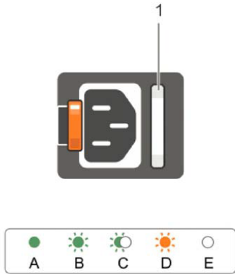
Figure 17: Power Supply unit Indicators
