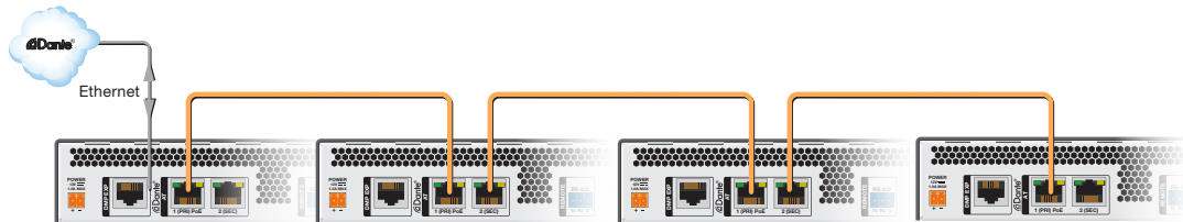
Figure 130. Daisy Chain Network Topology
