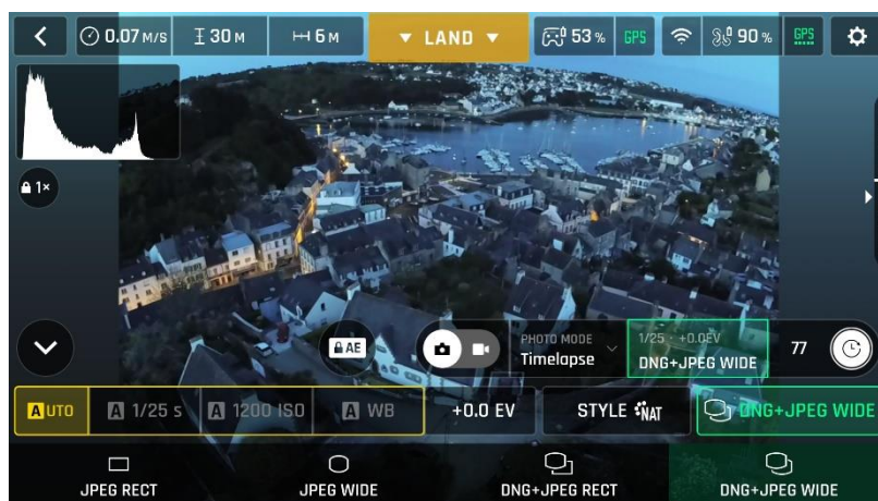
Android photo formats: DNG+JPEG WIDE (zoom is locked, stream image is WIDE)
