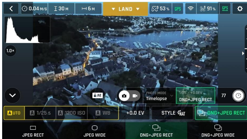
Android photo formats: DNG+JPEG RECT (zoom is unlocked, stream image is RECT)
