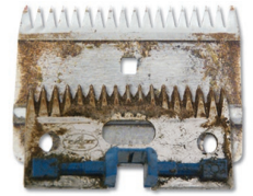
Example of dirty blades/light rust
