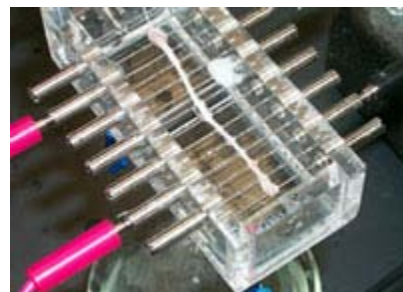
Ether swab alongside, but not touching, nerve. (Shown in Harvard Apparatus 50-720 nerve chamber.)
