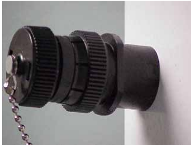
Fig. 13 Shorting Plug installed
