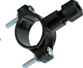
hole clean through both sides of the drainpipe. This will result in a leak, and require replacement of that piece of drainpipe. Mount the drain saddle clamp on top of the template with the holes aligned. You may use a screwdriver to align the holes. Fit drain saddle clamp back-plate and screws. Alternate tightening screws on each side of the drain saddle clamp to ensure an even, snug fit.
