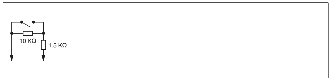
Figure 6.16 Resistor network for line fault detection
