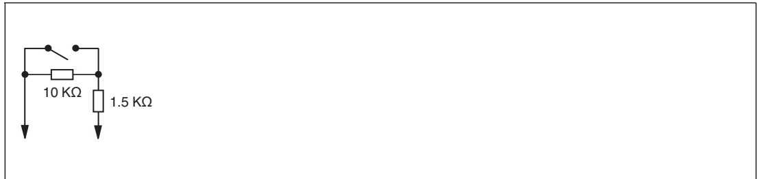
Figure 6.13 Resistor network for line fault detection
