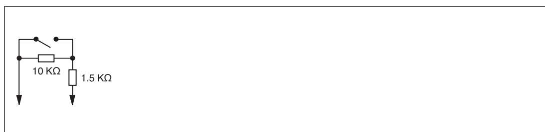
Figure 6.5 Resistor network for line fault detection
