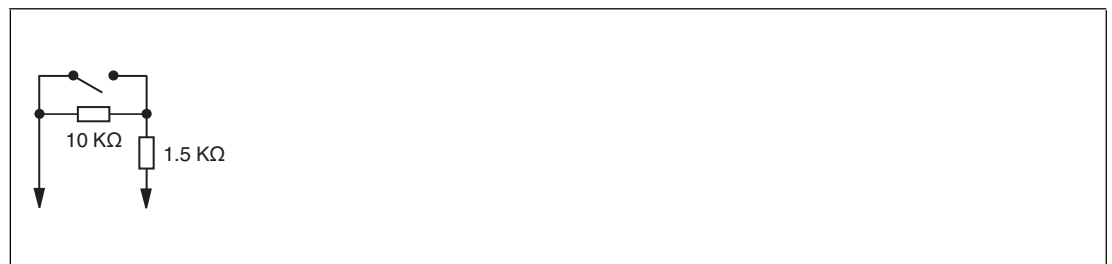
Figure 6.21 Resistor network for line fault detection
