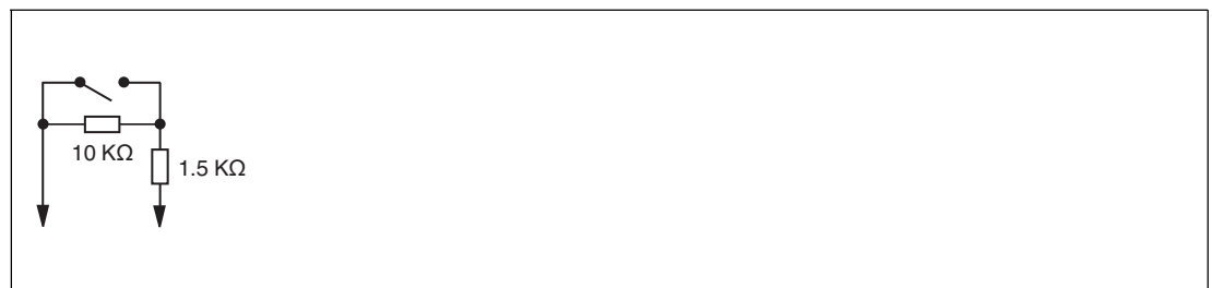
Figure 6.50 Resistor network for line fault detection
