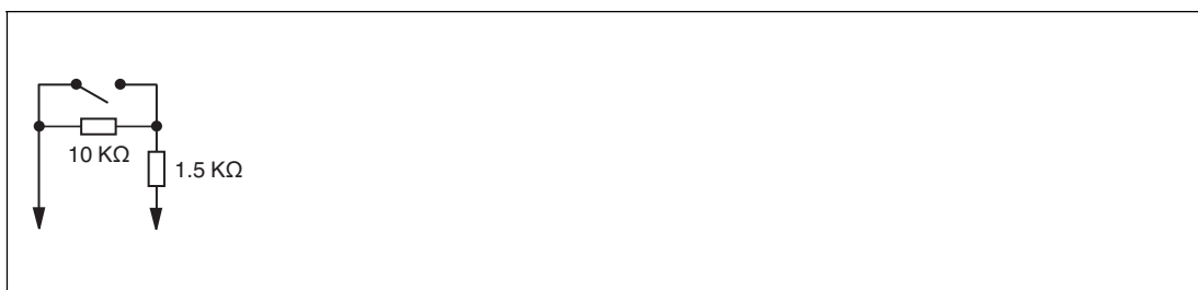
Figure 6.10 Resistor network for line fault detection
