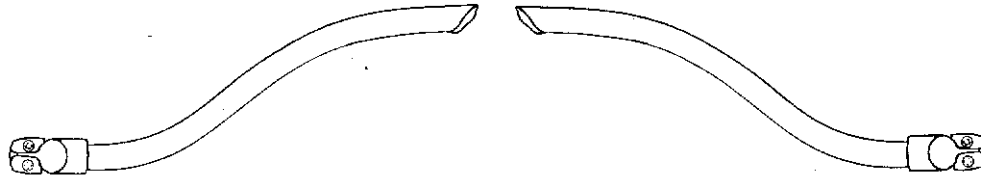
381736-01 Handle, exit, interior, wall, 32.50" 381736-02 Handle, exit, interior, dash, 20.50"
