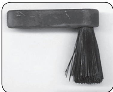
Level 2- Moderate splaying, have spare ready
