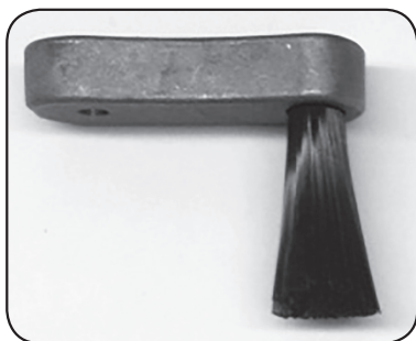
Level 1- New brush, minimal "splay"
