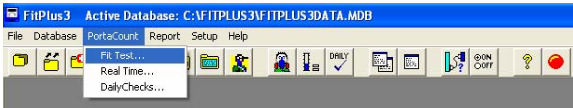
Figure 4-1. Starting a Fit Test When FitPlus is Already Running
