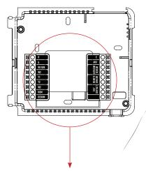
To remove the thermostat backplate: Gently separate the display from the base by pulling first from one side, then the other until the two pieces unsnap.
