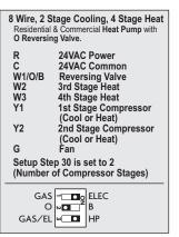
Note: When the unit goes into 4th stage heating, there is no 4th stage indicator, the display will still show 3rd stage.
