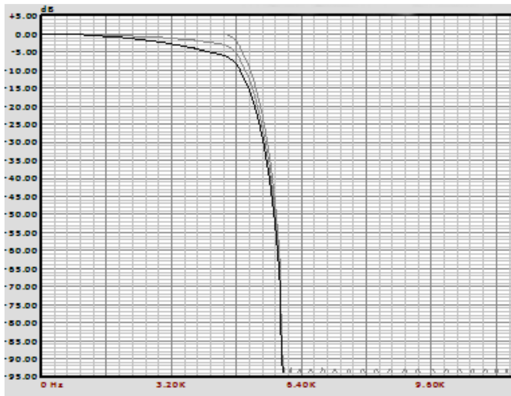
Figure 2-5: Effect of the LPF Shape Control with F = 5.0 kHz
